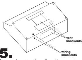
Remove knockout from the wiring opening (top or rear) to be used.
